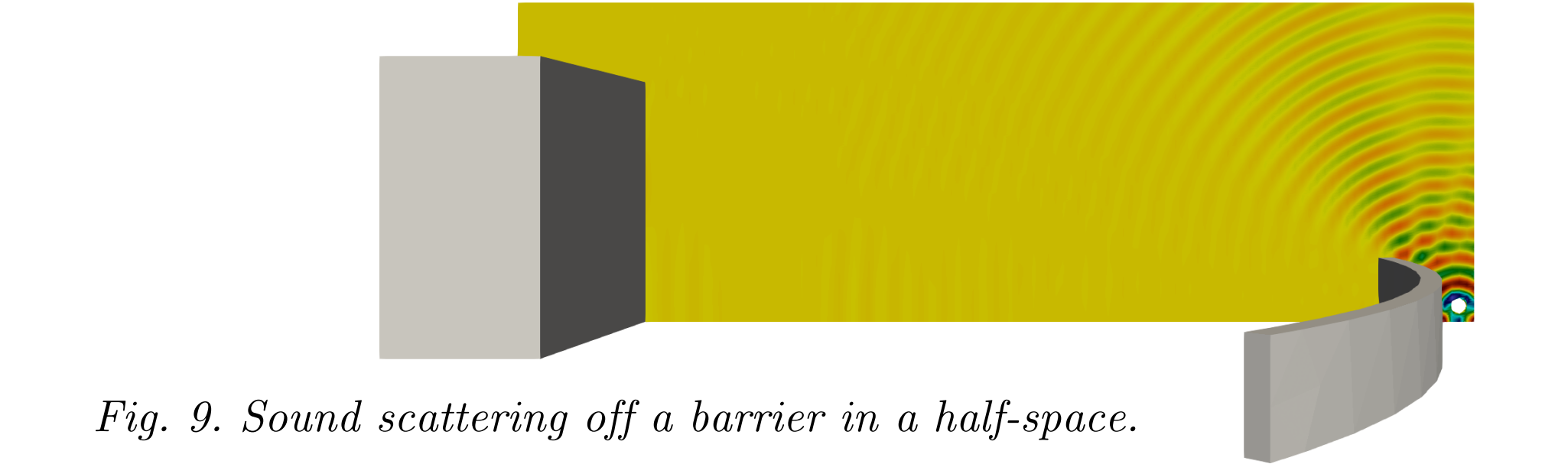
Fig. 9. Sound scattering off a barrier in a half-space.
