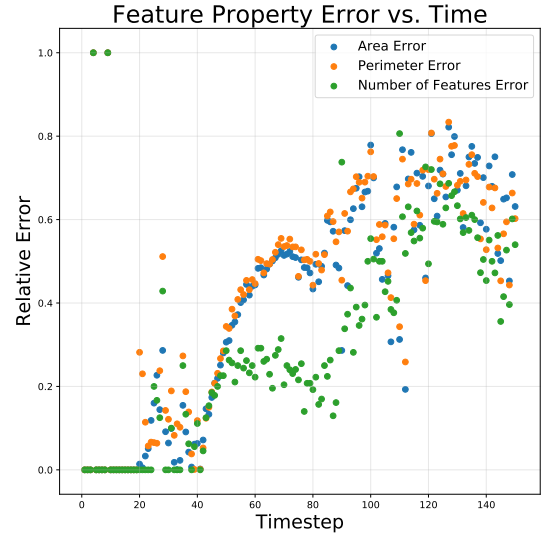
Fig. 7. Relative error (as compared to original, uncompressed data) for the specified properties over the course of an XGC simulation run compressed with SZ ( \text{rel}=0.1 ).
